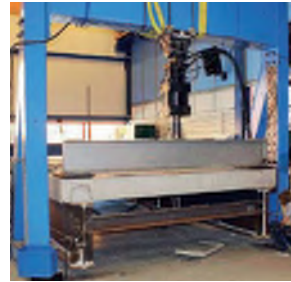
Fig. 5. Two point loads applied straight above the steel beams
