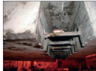
(b) The channel in one slab element used in laboratory testing
