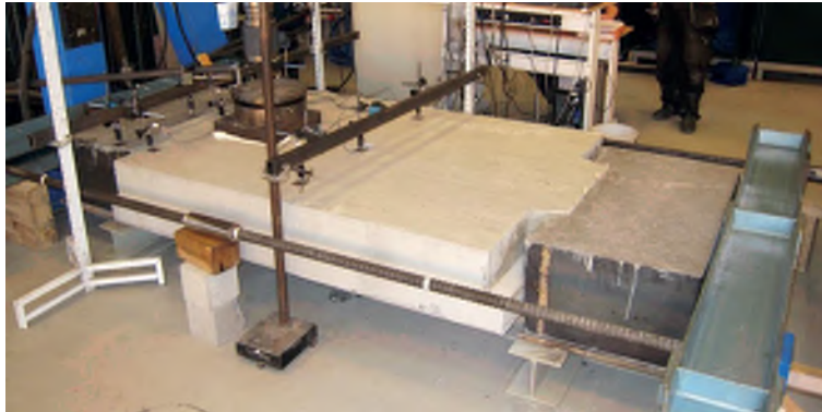
Figure 3.17 The shear key test set-up
