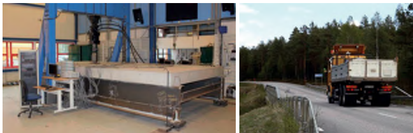
Figure 3.10 Large-scale laboratory test (left) and field monitoring of the Rokån Bridge (right)
